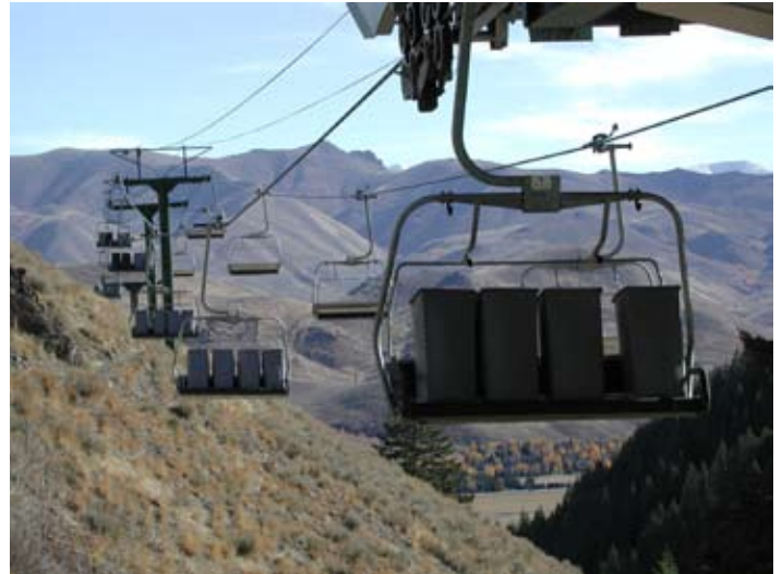
Testing a retrofit drive installation
